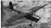
Built to perform a wide variety of utility liaison duties, Convair L-13 is a rugged craft designed to operate from unimproved fields. Powered by a 300-hp. Franklin engine a two-place, electrically controllable push prop. plane is rated to have a top speed of 119 mph at 2,900 ft. gross weight.
